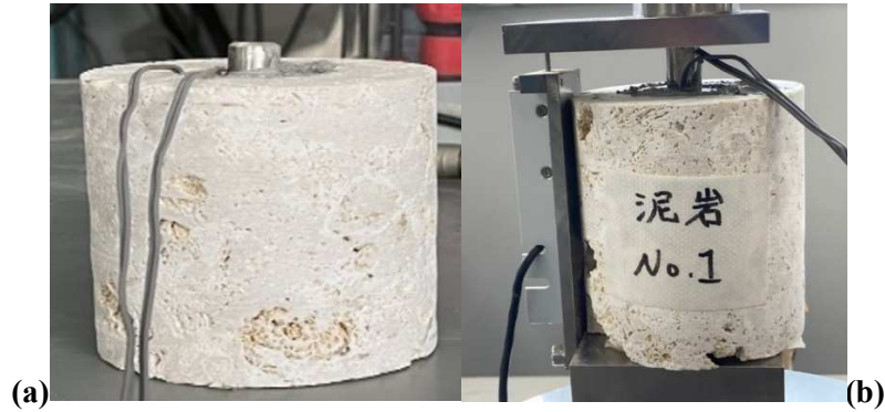
Figure 2. Views of samples for (a) static and (b) creep tests.
