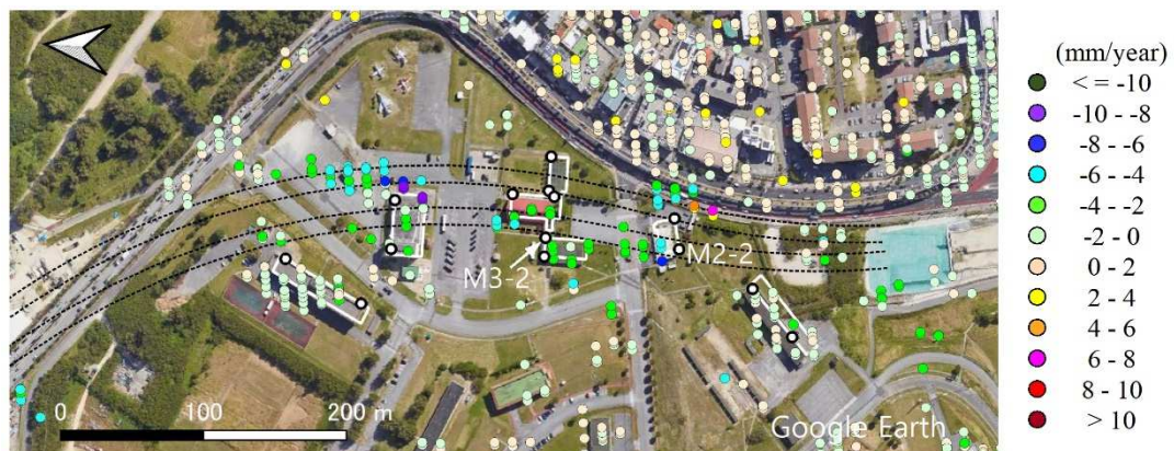
Figure 5. Distribution of LOS displacement velocity at PS points by PSI method with coherence less than 0.75 hidden.
